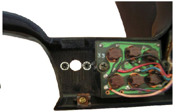
5. Insert Joystick board from the back and screw in (The Connector must be at the top)
