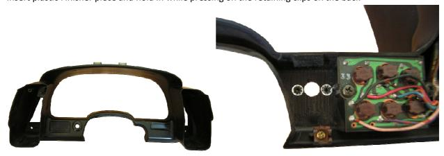
5. Insert Joystick board from the back and screw in (The Connector must be at the top)
